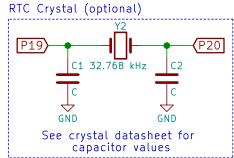
Figure 3 – External RTC crystal circuits
