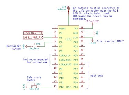
Figure 4 – Minimum required circuit
