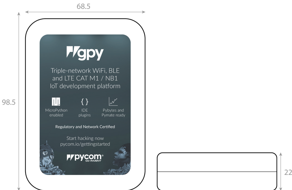
Figure 8 – Mechanical drawing of packaging – Units: mm
