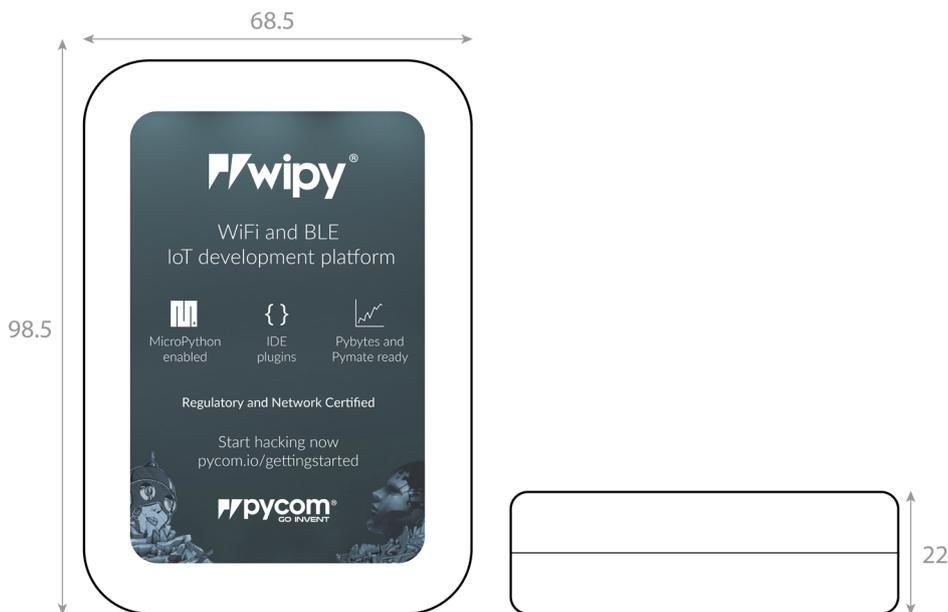
Figure 10 – Mechanical drawing of packaging – Units: mm
