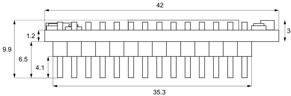
Figure 6 – Mechanical drawing (side view) – Units: mm
