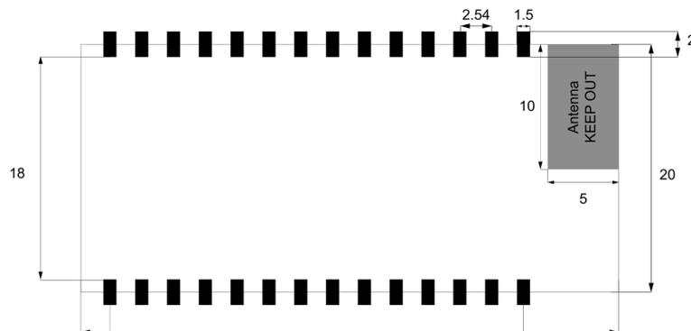
Figure 8 – Recommended land pattern (surface mount) – Units: mm
