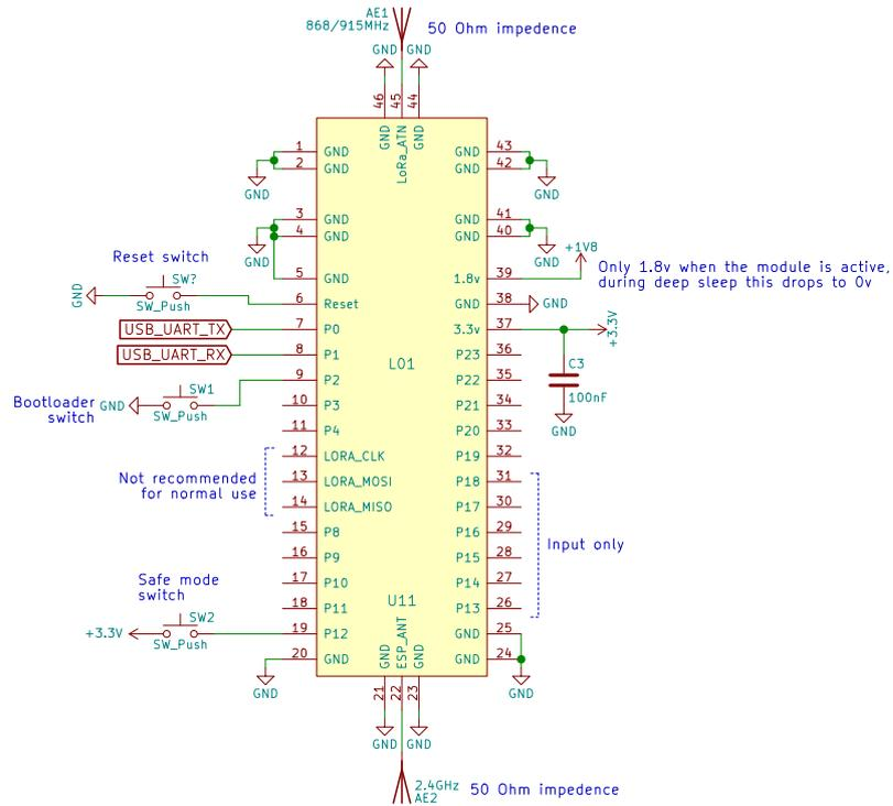
Figure 4 – Minimum required circuit
