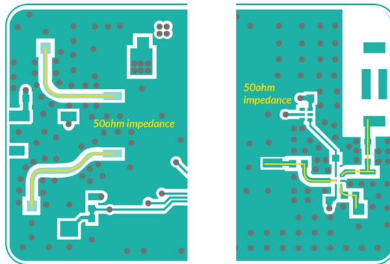
Figure 7 – 50-ohm impedance antenna connections
