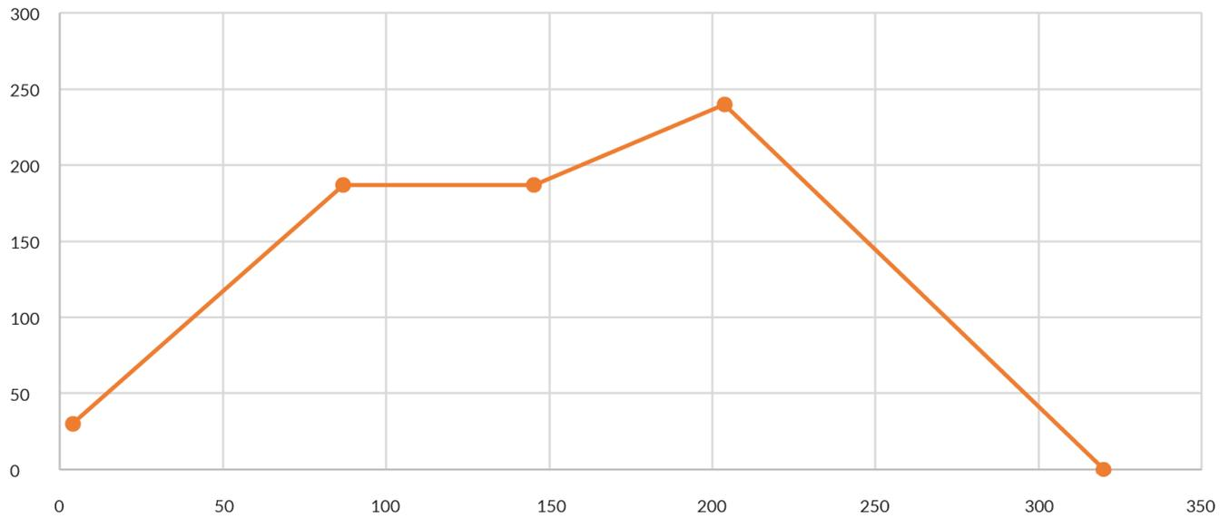
Figure 10 – Reflow soldering temperature profile
