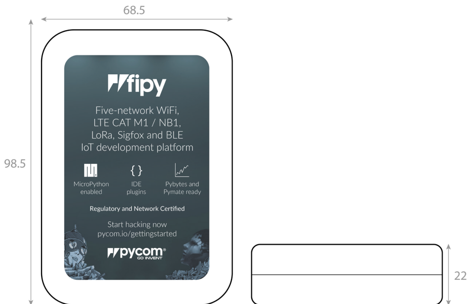
Figure 7 – Mechanical drawing of packaging – Units: mm
